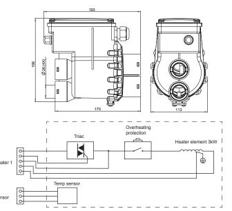
This whirlpool water heater is developed for private use and shall be installed and used indoors. The heater can be mounted on the pumps suction or pressure side.
